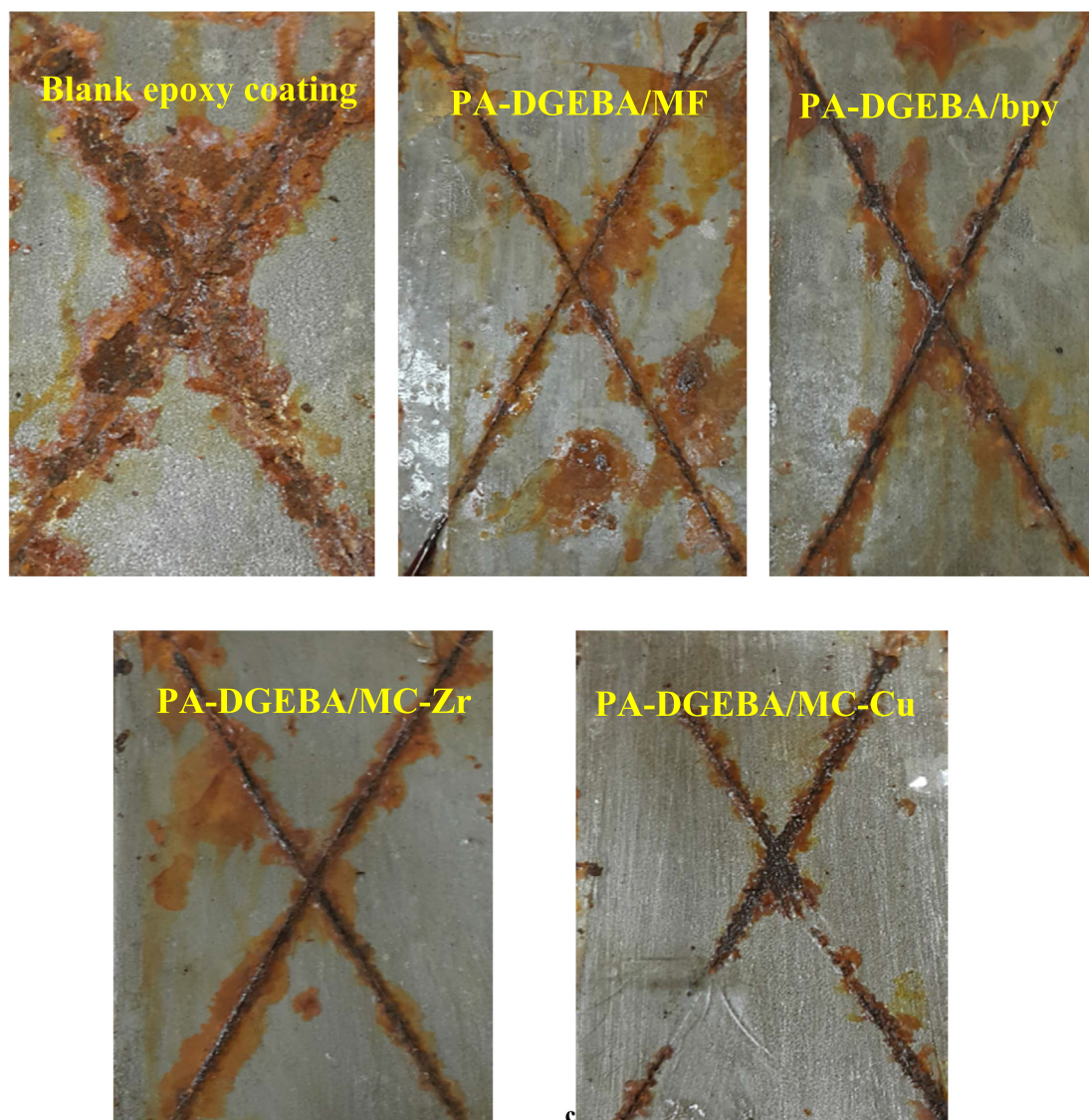
Fig. 7 Salt spray accelerated corrosion experiment for the investigated surface modified epoxy coated panels against blank unmodified coating after direct exposure to aggressive fog (5% NaCl solution and humidity of 95 at 35 °C).
