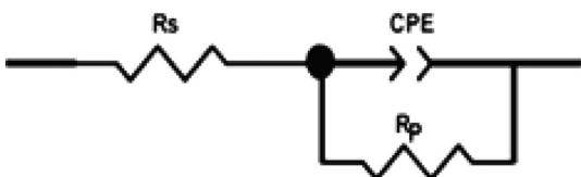
Fig. 6 Equivalent circuit used in experimental impedance fit.
