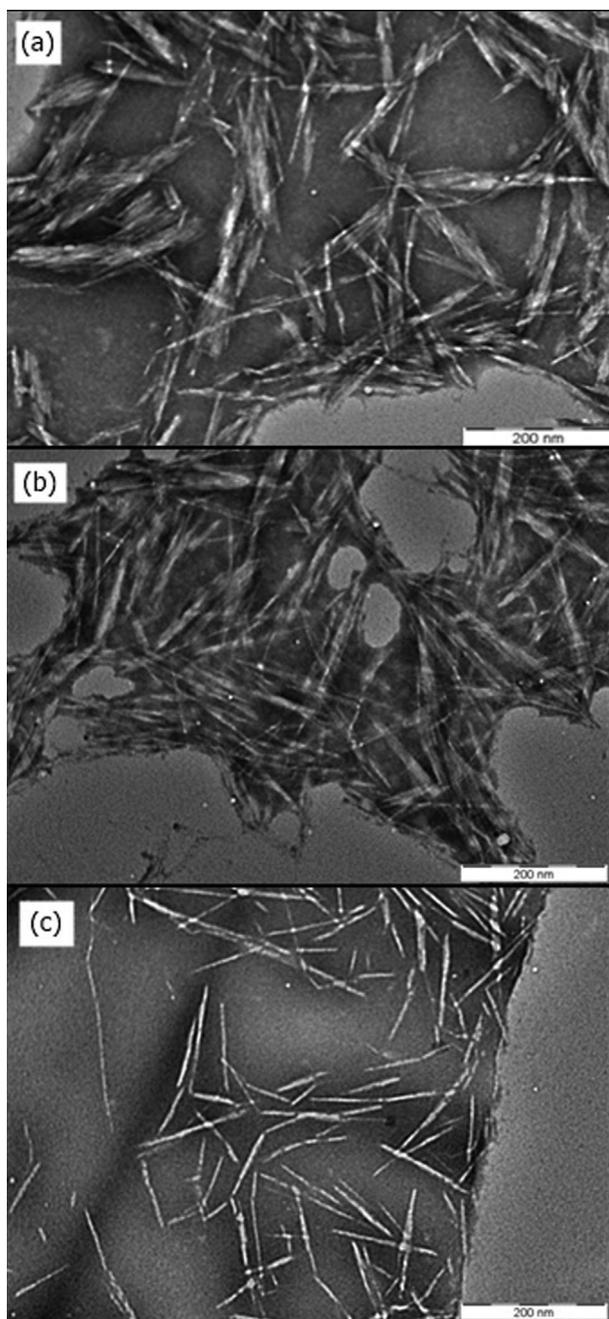
**Fig. 6** TEM images of microcrystalline cellulose, TEMPO-oxidized microcrystalline cellulose, and cellulose nanocrystals isolated from *Elaeis guineensis* empty fruit bunches. Adapted with permission from (Rohaizu and Wanrosli, 2017).
