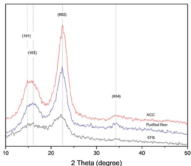
**Fig. 9** XRD analyses conducted on raw empty fruit bunches, fibres after a chemical pretreatment, and cellulose nanocrystals. Adapted with permission from (Foo et al., 2019).
