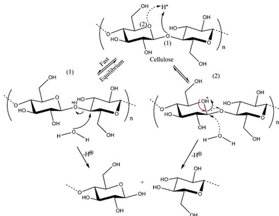
**Fig. 2** Mechanism of cellulose chain acid hydrolysis. Adapted with permission from (Kargarzadeh et al., 2017).
