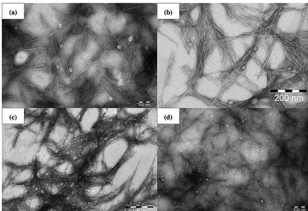
**Fig. 5** TEM images of (a) cellulose nanocrystals prepared by sulphuric acid hydrolysis, (b) Cellulose nanocrystals prepared by combination of formic acid and hydrochloric acid hydrolysis, (c) Cellulose nanocrystals prepared by formic acid hydrolysis and (d) Cellulose nanocrystals prepared by TEMPO-mediated oxidation. Adapted with permission from (Li et al., 2015).
