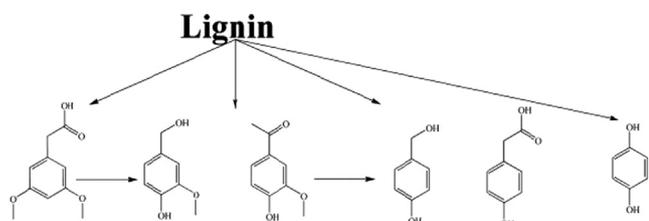
**Fig. 1** Fragmentation of lignin structure during hydrothermal pretreatment. Adapted with permission from (Gao et al., 2016).
