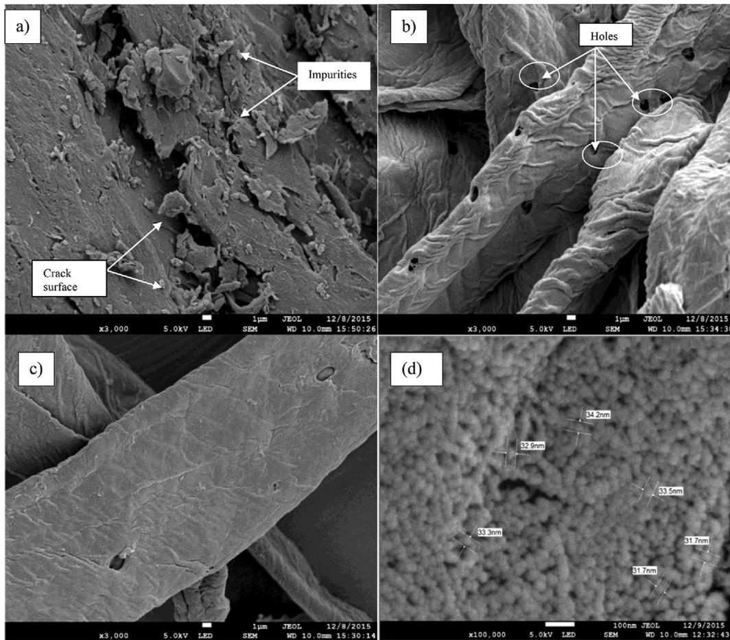
**Fig. 7** FESEM images of raw empty fruit bunches, empty fruit bunch pulp, alkaline-treated empty fruit bunch pulp, and cellulose nanocrystals. Adapted with permission from (Zianor Azrina et al., 2017).
