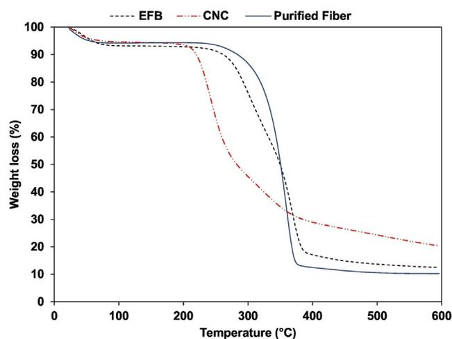
Fig. 11 Weight losses of empty fruit bunches (EFB), pre-treated empty fruit bunches (purified fibre) and cellulose nanocrystals isolated from empty fruit bunches (CNC). Adapted with permission from (Foo et al., 2019).
