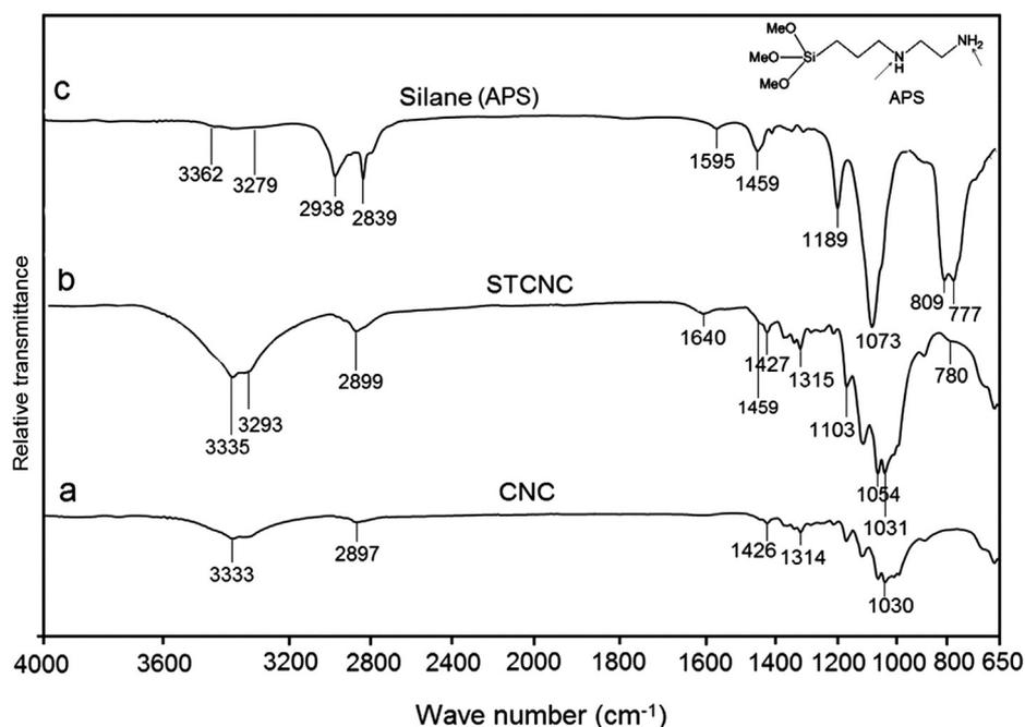
**Fig. 10** Sample of FTIR spectra of cellulose nanocrystals produced by different treatments. Adapted with permission from (Kargarzadeh et al., 2015).
