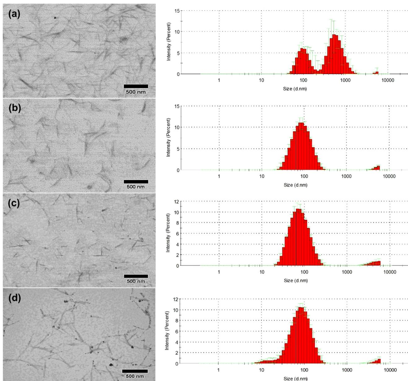
**Fig. 8** FESEM images and particle size distribution charts of cellulose nanocrystals produced from (a) 56 wt% of  $\text{H}_2\text{SO}_4$ , A/P 15, 30 min, (b) 58 wt% of  $\text{H}_2\text{SO}_4$ , A/P 15, 45 min, (c) 60 wt% of  $\text{H}_2\text{SO}_4$ , A/P 15, 30 min, and (d) 57.88 wt% of  $\text{H}_2\text{SO}_4$ , A/P 20, 60 min. Adapted with permission from (Foo et al., 2020).
