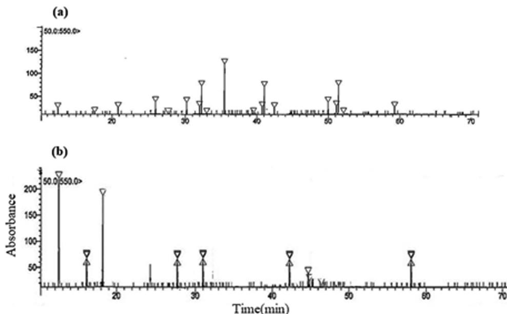
**Fig. 4** HPLC charts for separation of amino acids (a) non-essential and (b) essential present within Licorice root extract.
