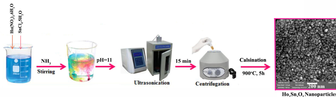
Scheme 1. Schematic diagram of fabrication process of Ho_2Sn_2O_7 .
