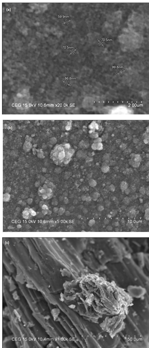
**Fig. 2** SEM images of (a, b) CeO<sub>2</sub>/Au/GO nanocomposite and (c, d) Au/GO nanocomposite.
