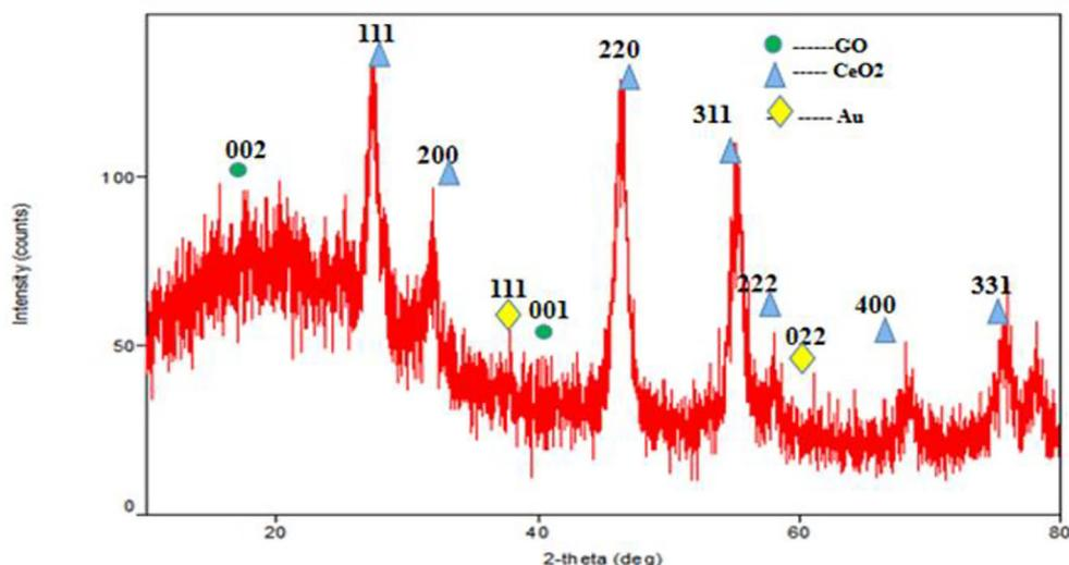
Fig. 1 XRD Analysis of CeO<sub>2</sub>/Au/GO Nanocomposites.
