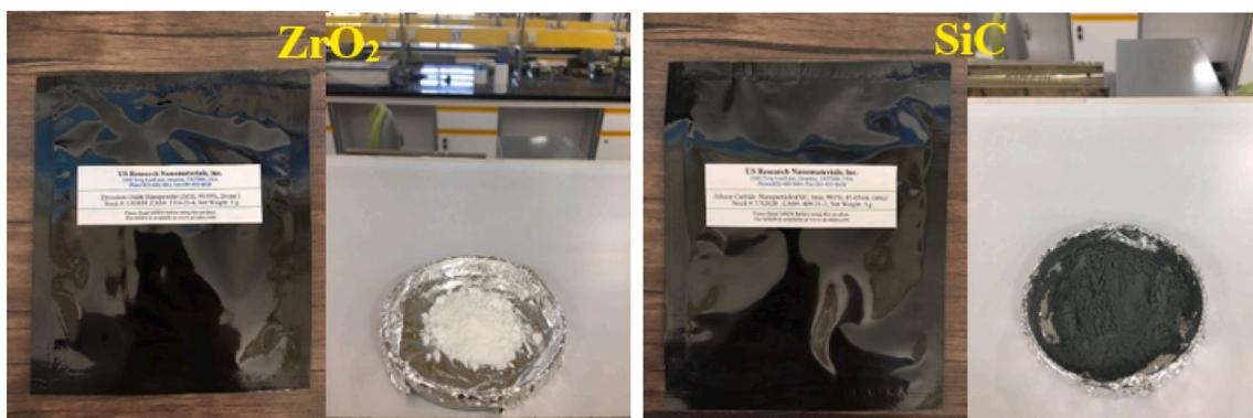
Fig. 1. Images of ZrO<sub>2</sub> and SiC nanoparticles.
