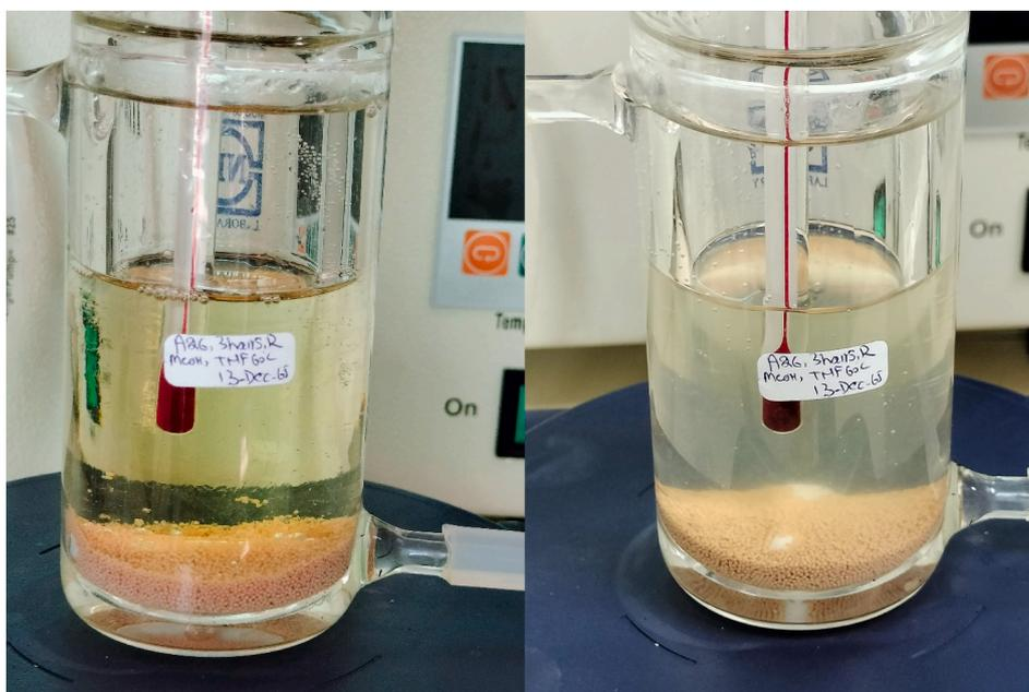
**Fig. 12.** Photographs of the reaction mixtures in the reactor before (left) and after (right) 3 h transesterification with A26. The white balance and tint of the photograph on the left were adjusted to achieve a natural appearance.
