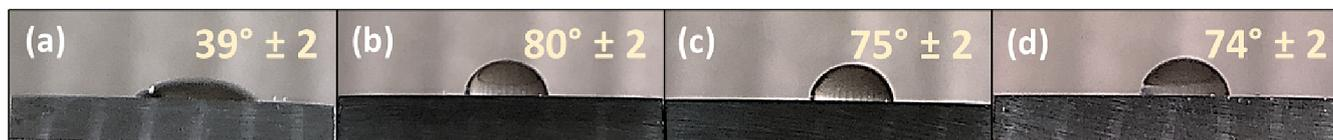
Fig. 9. WCAs of (a) bare substrate, (b) neat PVDF, (c) MLDH@PVDF, (d) and ZLDH@PVDF composite coatings.
