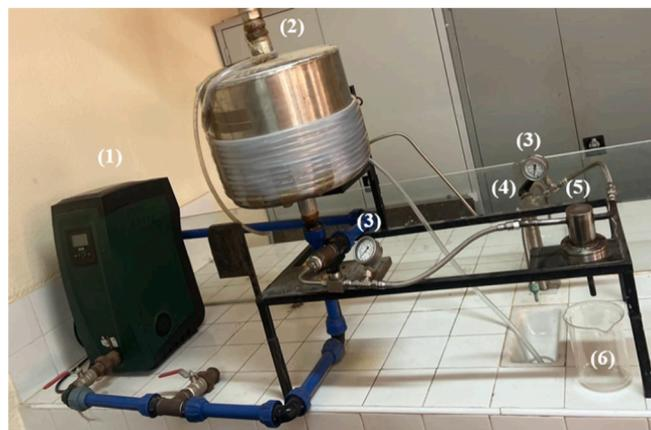
Fig. 1. Diagram of the laboratory pilot (1: pump, 2: solution tank, 3: pressure manometer, 4: valve, 5: sample holder module, 6: filtrate).
