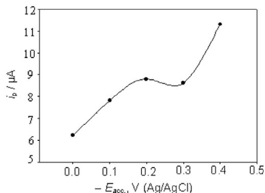
**Figure 3** Effect of deposition potential on  $5 \times 10^{-5}$  mol  $L^{-1}$  secnidazole in BR buffer solution of pH 5.3 at  $t_{acc} = 60 \text{ s}$ ,  $t = 500 \text{ mV s}^{-1}$  and step height = 5 mV.
