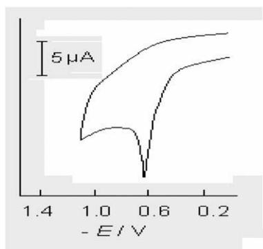
**Figure 2** Cyclic voltammogram of  $1 \times 10^{-4}$  mol  $L^{-1}$  secnidazole in BR buffer at pH 7.34 at scan rate of  $500 \text{ mV s}^{-1}$ .
