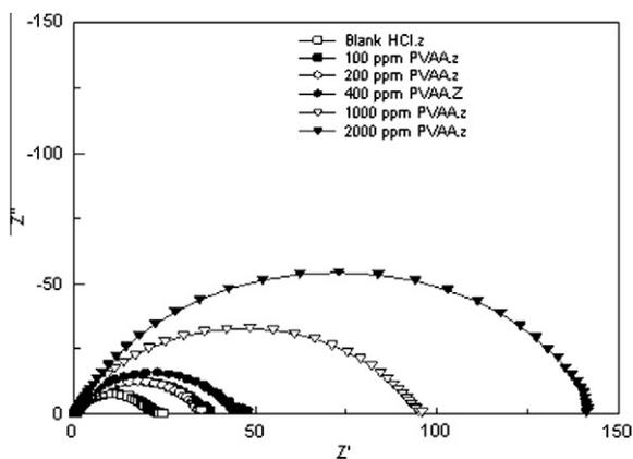
**Figure 5** Nyquist plots of mild steel in 1.0 M HCl.
