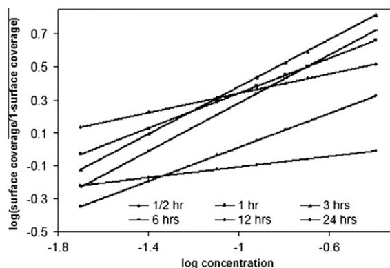
**Figure 2** Langmuir's adsorption plots of PVAA composite in 1.0 M HCl.
