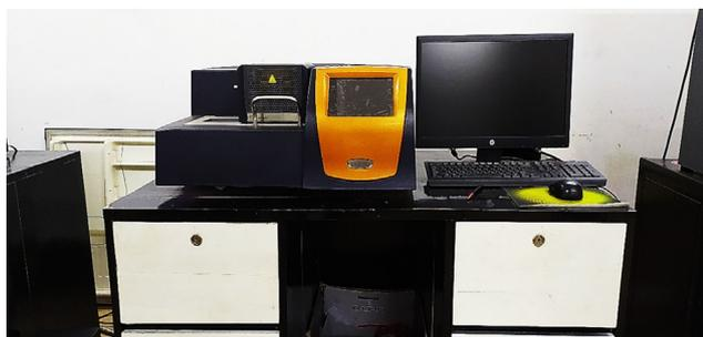
**Fig. 4** TGA setup for determination of decomposition temperature.
