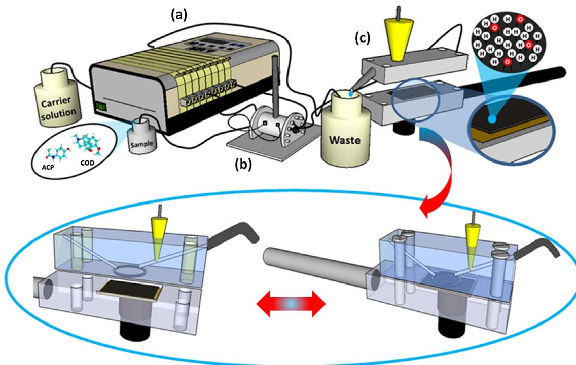
**Figure 1** Schematic representation of the flow injection analysis (FIA) system employed: (a) peristaltic pump, (b) manual injector and (c) electrochemical detector with an Ag/AgCl ( $3.0 \text{ mol L}^{-1} \text{ KCl}$ ) electrode as the reference electrode, a stainless steel tube as the auxiliary electrode and a CP-BDD electrode as the working electrode.
