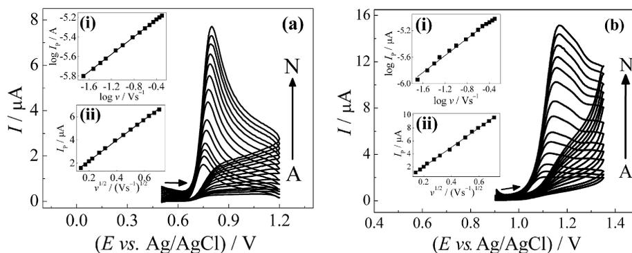
**Figure 3** Cyclic voltammograms obtained for a 0.2 mol L<sup>-1</sup> phosphate buffer (pH 4.0) solution containing (a) ACP 10.0 μmol L<sup>-1</sup> and (b) COD 10.0 μmol L<sup>-1</sup> using a CP-BDD electrode at different scan rates: 20 (A); 30 (B); 40 (C); 50 (D); 75 (E); 100 (F); 150 (G); 200 (H); 250 (I); 300 (J); 350 (K); 400 (L); 450 (M); and 500 (N). Insets: (i)  $\log I_p$  vs.  $\log v$  curves and (ii)  $I_p$  vs.  $v^{1/2}$  curves.
