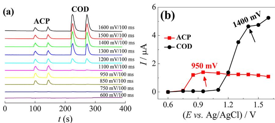
**Figure 4** (a) Amperograms obtained in FIA-MPA system after single injections of supporting electrolyte solutions containing ACP 10.0 μmol L<sup>-1</sup> or COD 10.0 μmol L<sup>-1</sup>. (b) Hydrodynamic voltammograms obtained for ACP and COD by plotting the values of peak current as a function of the corresponding applied potential pulses. Supporting electrolyte: 0.05 mol L<sup>-1</sup> H<sub>2</sub>SO<sub>4</sub>; injection volume: 350.0 μL and flow rate: 3.8 mL min<sup>-1</sup>.
