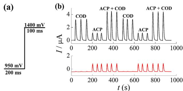
**Figure 5** (a) MPA waveform applied to the CP-BDD electrode vs. potential pulse time. (b) FIA-MPA response for injections in triplicate of supporting electrolyte solutions containing only ACP (10.0 μmol L<sup>-1</sup>), only COD (10.0 μmol L<sup>-1</sup>) or ACP + COD (both at 10.0 μmol L<sup>-1</sup>). Supporting electrolyte: 0.05 mol L<sup>-1</sup> H<sub>2</sub>SO<sub>4</sub>; injection volume: 350.0 μL and flow rate: 3.8 mL min<sup>-1</sup>.
