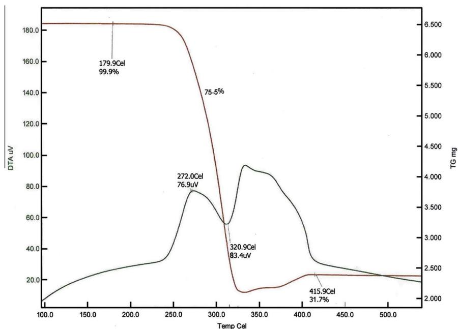
Figure 2 TG/DTA spectrum of Co(II) complex.
