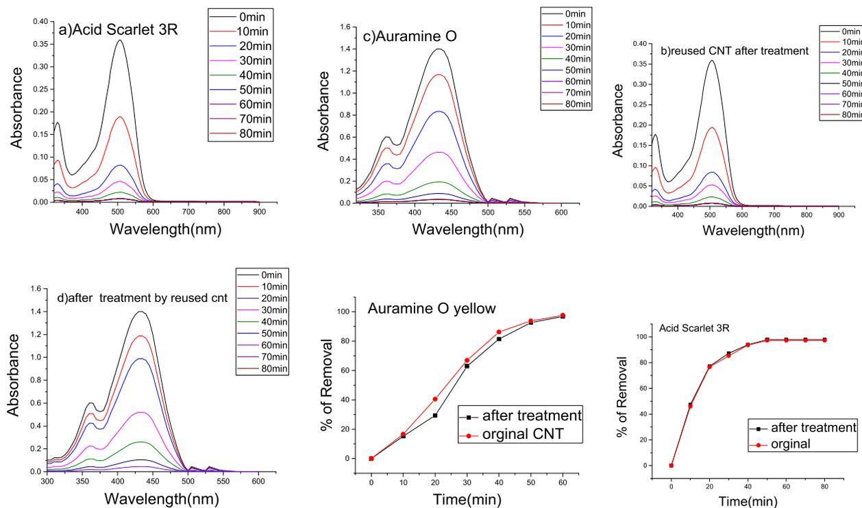
Fig. 9 Regeneration of MWNTs adsorbent.
