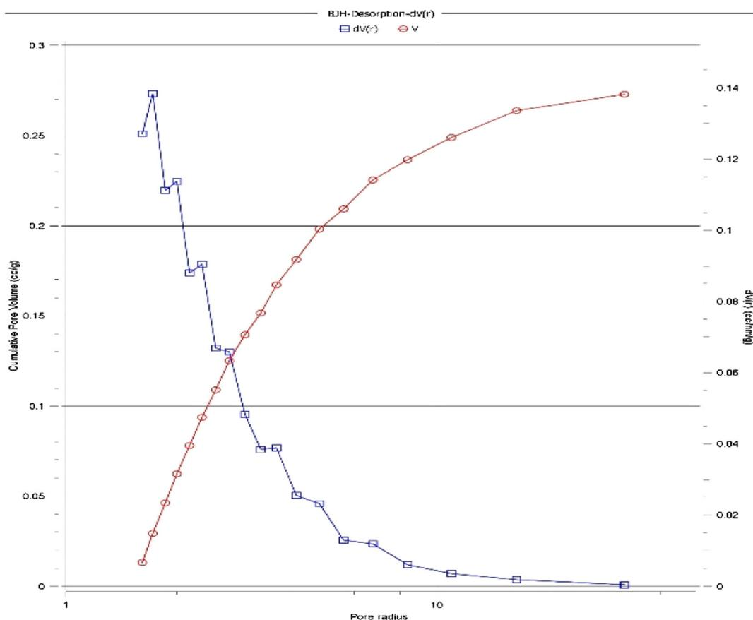
Fig. 4b Pore size measurements of MWNTs.
