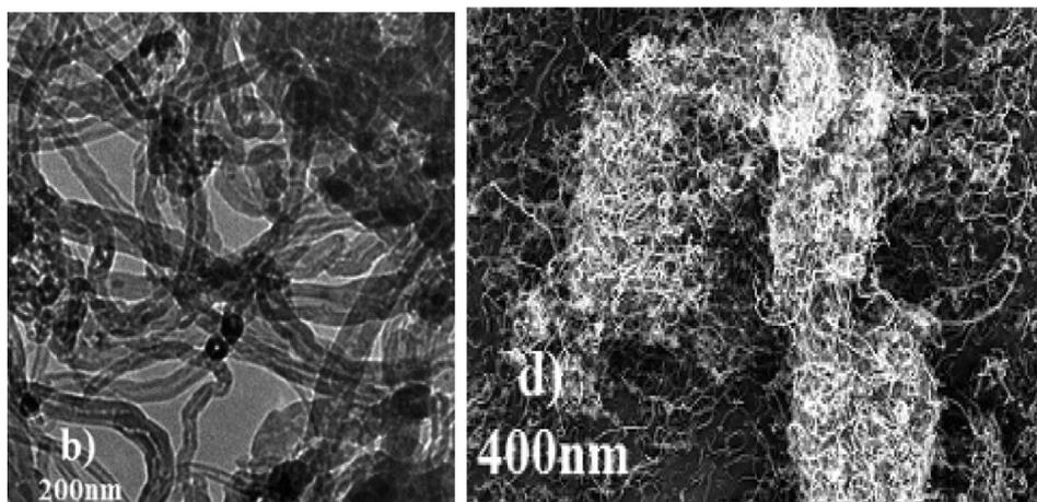
Fig. 2b and 2d TEM and SEM images of MWNTs after adsorption of dyes.
