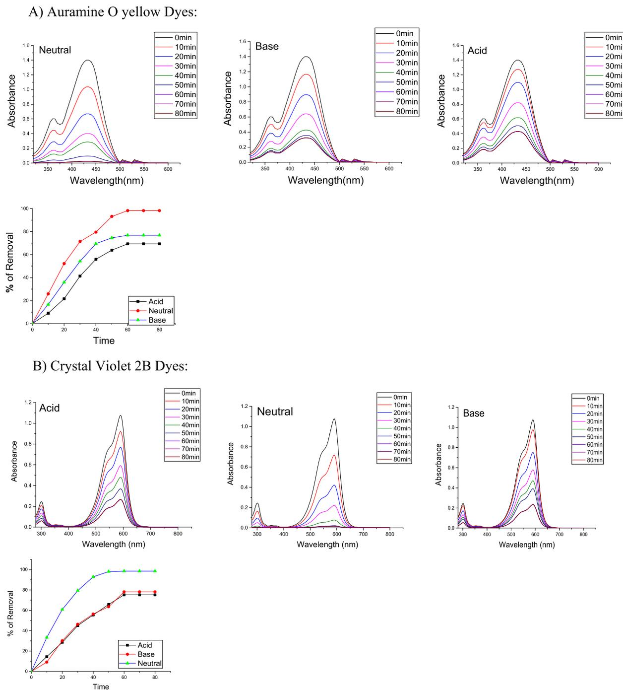
**Fig. 8** Effect of pH on dyes removal (a) acid scarlet 3R, (b) auramine O yellow and (c) crystal violet 2B under optimum conditions of initial dyes concentration 10 mg/L, time 60 min, adsorbent doe 40 mg and 240 rpm.
