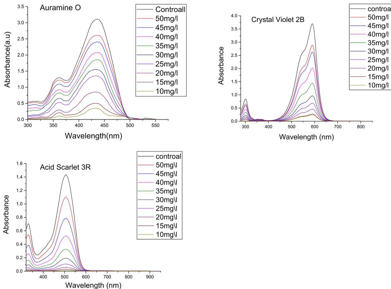
**Fig. 7** Effect of dyes concentrations under optimum experimental conditions of pH 7,  $t = 50$  min, MWNTs dose of 40 mg and 240 rpm.
