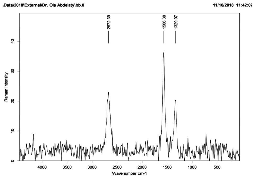
Fig. 3a Raman spectrum of MWNTs before adsorption of dyes.
