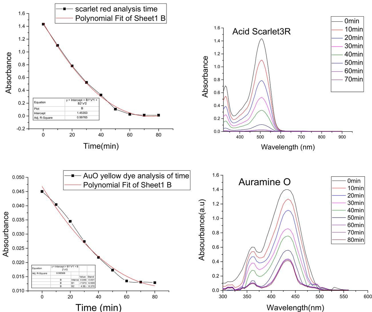
**Fig. 6** The effect of contact time on removal of dyes with constant concentration at the presence of constant dose of MWNTs and constant agitation speed at 50 min.
