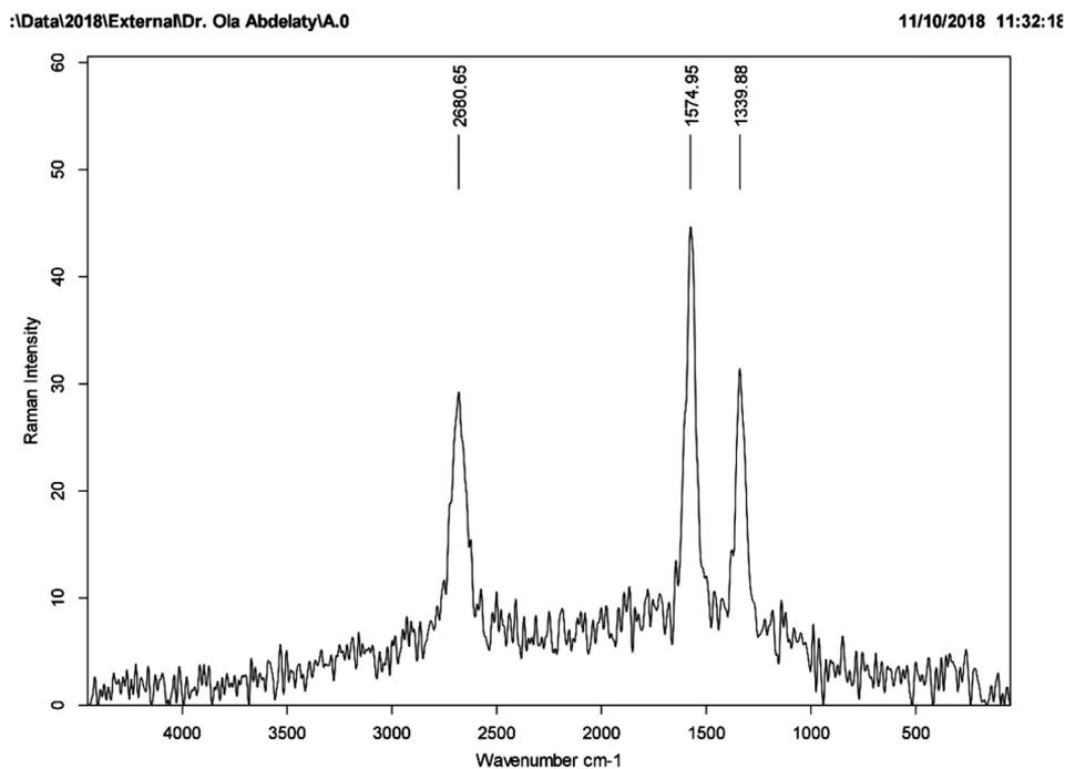
Fig. 3b Raman spectrum of MWNTs after adsorption of dyes.
