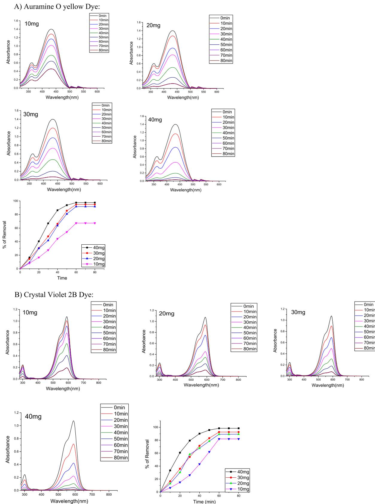
**Fig. 5a-c** Removal of three dyes using different doses of MWNT through 80 min of constant time, 240 rpm of agitation speed and 10 mg/l of dyes concentration.
