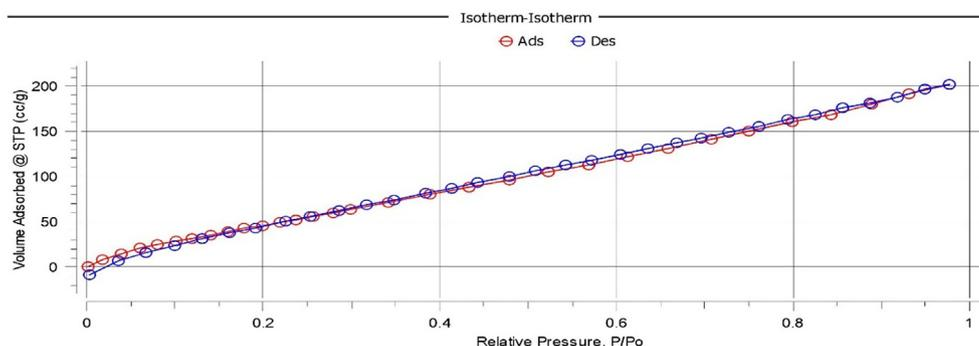
Fig. 4a BET surface area of MWNTs (a)  $N_2$  adsorption–desorption isotherm based surface area measurement.
