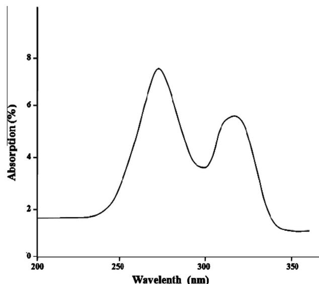
Figure 1 Electronic spectra of *p*-HBBF terpolymer resin.
