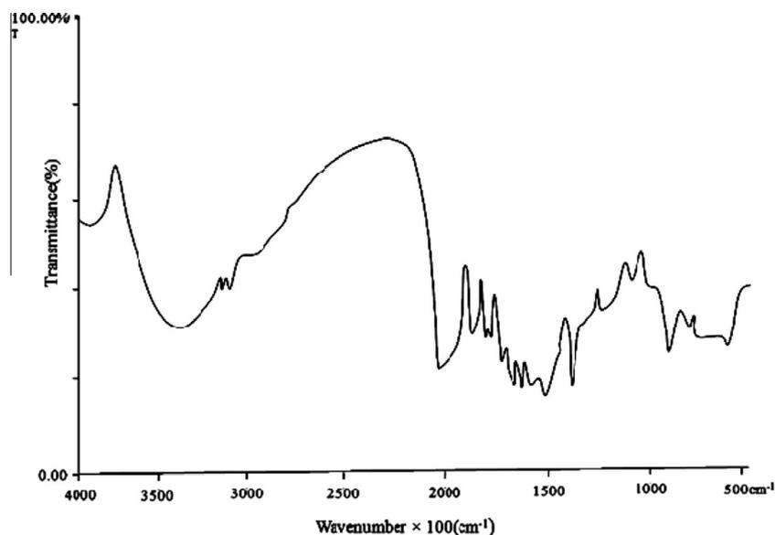
Figure 2 Infrared spectrum of *p*-HBBF terpolymer resin.
