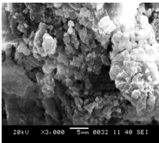
Figure 5 SEM micrographs of *p*-HBBF terpolymer resin at 3000 $\times$  magnification.
