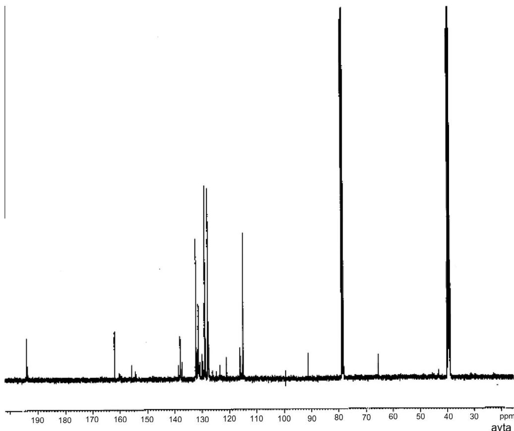
Figure 4  $^{13}\text{C}$  NMR spectra of *p*-HBBF terpolymer resin.
