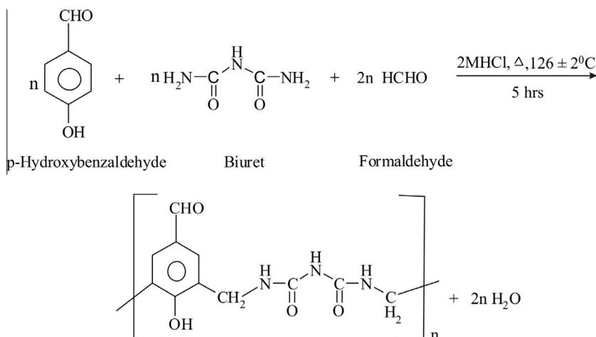
**Scheme 1** Synthesis and suggested structure of *p*-HBBF terpolymer resin.
