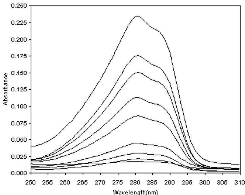
**Figure 2** UV spectrum of 17  $\beta$ -estradiol (0.5, 1, 1.5, 2, 4, 6, 8, 10 and 12  $\mu\text{g mL}^{-1}$ ).
