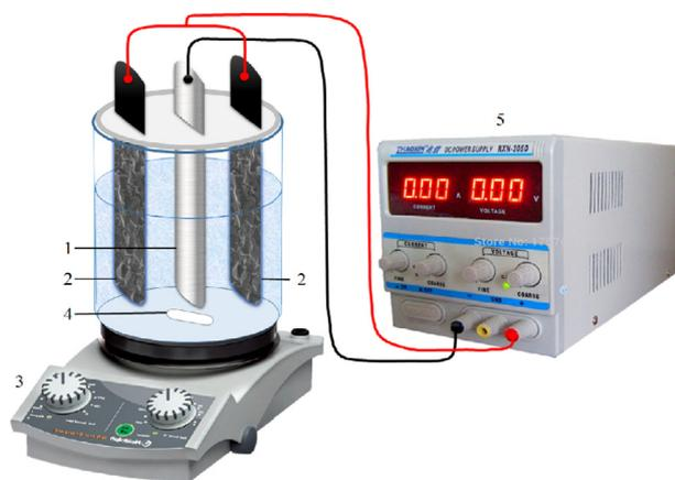
**Fig. 1** Schematic of the experimental setup (1. SS316 cathode, 2. G/β-PbO<sub>2</sub> anodes, 3. Magnetic stirrer, 4. Magnet, 5. DC power supply).
