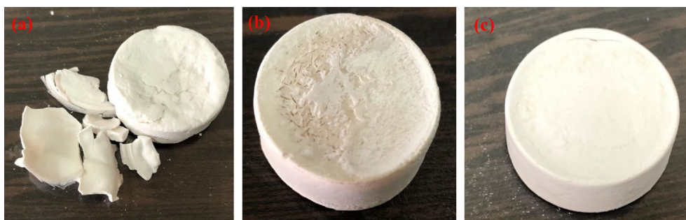
Fig. 1 Schematic of as-prepared samples CA-X/ZnO-Y aerogel with different weight ratios of MCC. a) 3 wt%, b) 6 wt% and c) 9 wt%.
