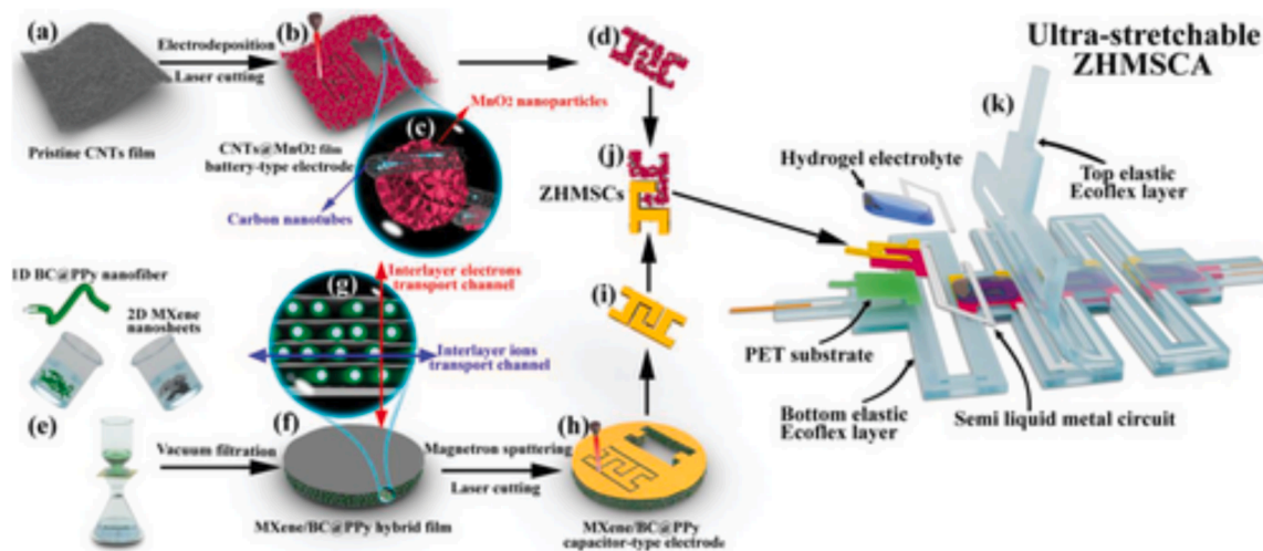
Fig. 10. An illustration of the ZHMSCA's ultra-stretchable production process (a) A pure carbon nanotube (CNT) film with randomly oriented carbon nanotubes; (b) \text{MnO}_2 nanoparticles electrodeposited on the CNTs film surface towards the CNTs@ \text{MnO}_2 hybrid film, which was then laser-cut into an interdigital CNTs@ \text{MnO}_2 battery-type electrode; (c) Following vacuum filtration, a blend of two-dimensional MXene nanosheets and one-dimensional BC@PPy nanofibers was generated; (f) MXene/BC@PPy hybrid film, which was then laser-cut into an electrode that resembled an interdigital capacitor; (j) ZHMSC was assembled; (k) The zoomed schematic diagrams of the microstructure; the ultra-stretchable ZHMSCA's decomposition diagram (c, g) (Cheng et al., 2021).
