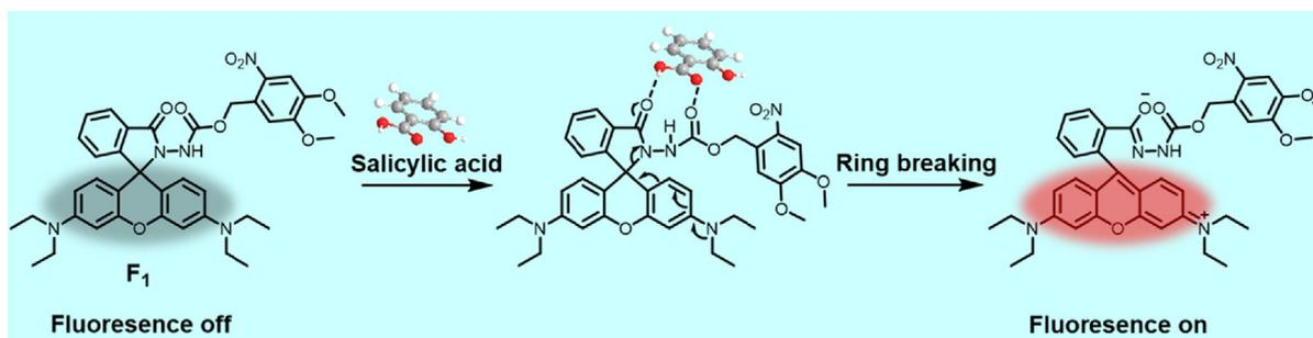
Fig. 9 Proposed mechanism for sensing SA using probe  $F_1$ .
