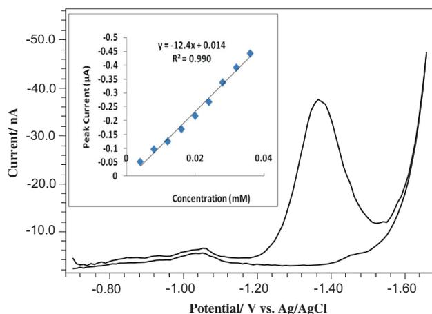
**Figure 3** Differential pulse adsorptive stripping voltammogram of pyruvic acid (0.004 mM) in 0.1 M ammonia buffer and 4 mM CTAB (pH  $8.2 \pm 0.01$ ) at HMDE, pulse amplitude  $-50$  mV, scan rate  $30$  mVs $^{-1}$ , current range  $10$   $\mu$ A, accumulation time  $30$  s.
