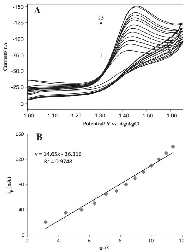
**Figure 1** (A) The CVs of 0.004 mM pyruvic acid in the ammonia buffer of pH  $8.2 \pm 0.01$  at HMDE, current range  $10 \mu\text{A}$ . scan rates ( $\text{mVs}^{-1}$ ) (1) 10, (2) 20, (3) 30, (4) 40, (5) 50, (6) 60, (7) 70, (8) 80, (9) 90, (10) 100 (11) 110, (12) 120 and 130. (B) Relationship between peak current ( $i_p$ ) versus root of scan rate ( $v^{1/2}$ ).
