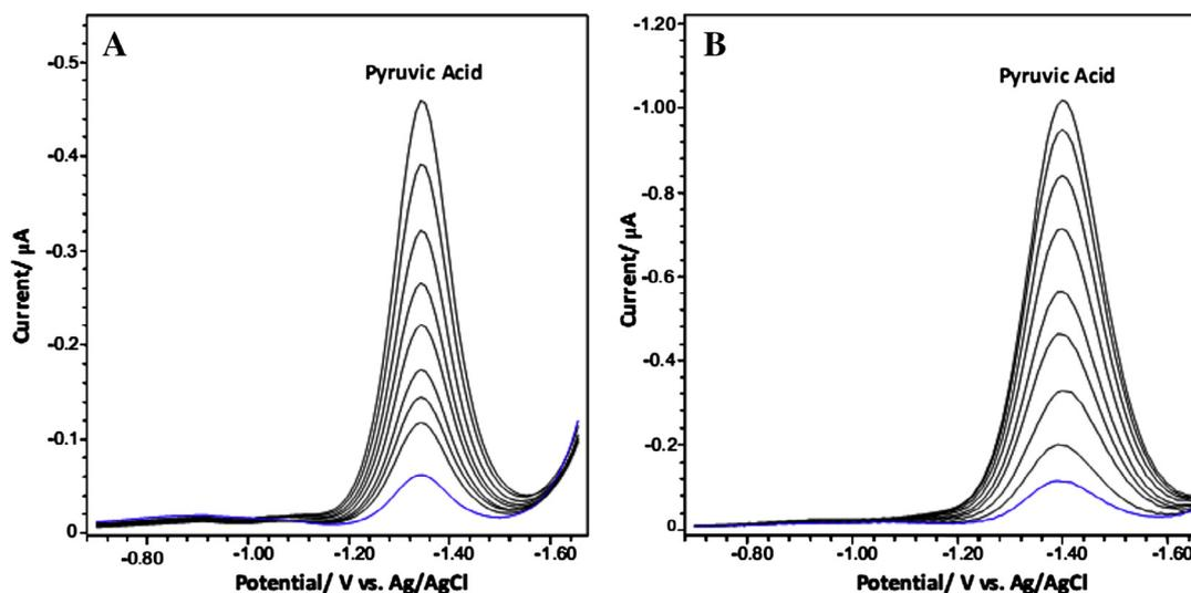
**Figure 5** Voltammograms of pyruvic acid using (A) DPAdSV and (B) SWAdSV at different concentrations including: (1) 0.004 (2) 0.008 (3) 0.012 (4) 0.016 (5) 0.02 (6) 0.024 (7) 0.028 (8) 0.032 (9) and 0.036 mM, pH 8.2, accumulation potential  $-0.5$  V, accumulation time 30 s.
