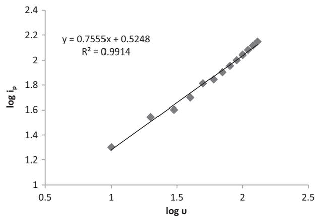
**Figure 2** Relationship between log of peak current ( $\log i_p$ ) versus log of scan rate ( $v$ ).
