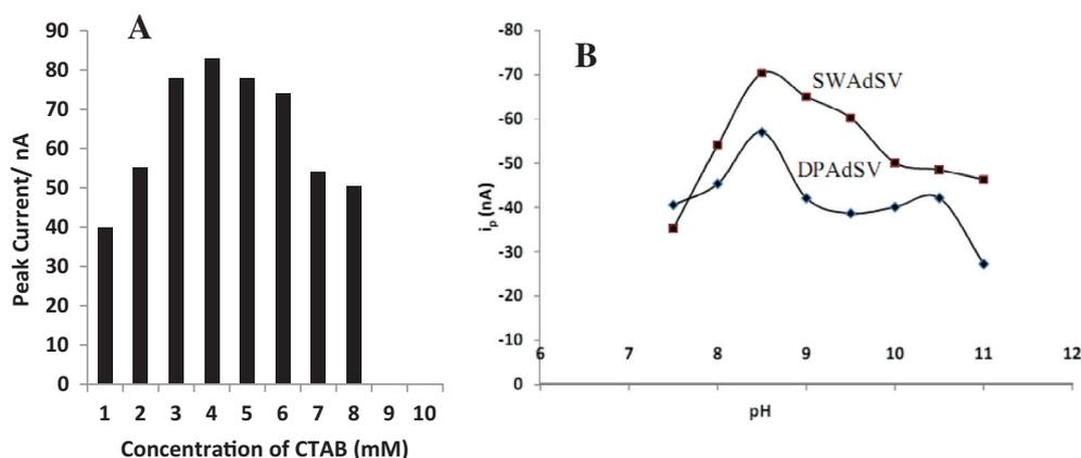
**Figure 4** (A) Plot of square wave adsorptive peak current vs. concentration of CTAB in ammonia buffer, pH  $8.2 \pm 0.01$ . (B) Influence of pH on the peak current response (using DPAdSV and SWAdSV) for 0.004 mM pyruvic acid in ammonia buffer (pH 7.5–11) and 4 mM CTAB after 30 s pre-concentration time; frequency ( $f$ ) = 20 Hz, and pulse amplitude = 50 mV at  $E_{acc} = -0.5$  V.
