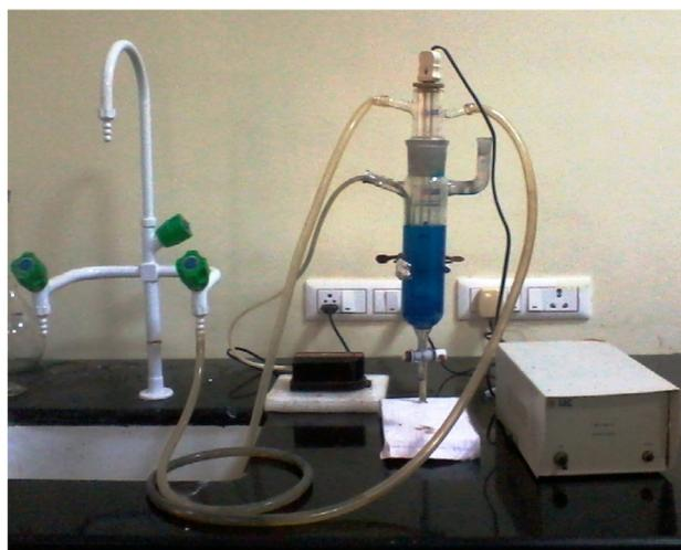
**Figure 5** Schematic and photographic images of photocatalytic reactor (reactor in OFF condition for visibility of reactor parts).
