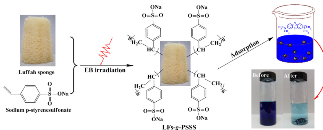
Scheme 1 Schematic of LFs-PSSS preparation by using electron beam radiation.
