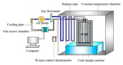
Figure 2. Sealed oxidation experimental apparatus.
