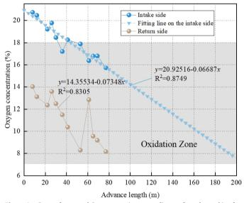
Figure 6. Curve of measured  $\rm O_2$  concentration versus distance from the working face in the goaf.
