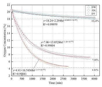
Figure 7. Oxygen concentration versus time curve. DY: Dayan, JDL: Jiudaoling, DW: Duanwang.
