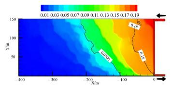
Figure 5. Initial O<sub>2</sub> concentration distribution.
