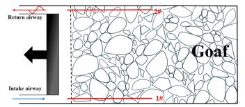
Figure 3. Tube bundle layout diagram.
