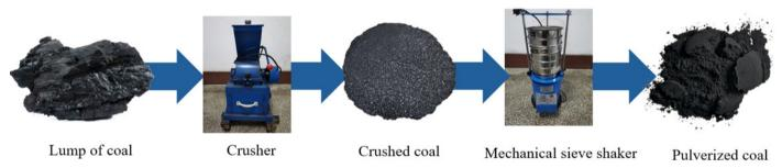
Figure 1. Coal sample preparation process.
