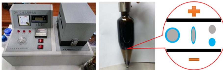
Fig. 3 Demulsifier selector and its electrical separation mechanism.
