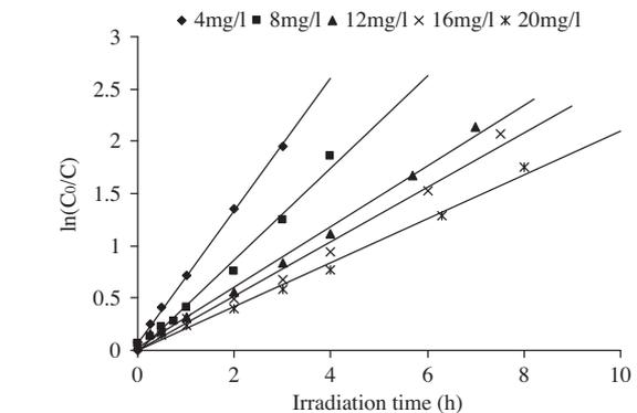
**Figure 4** Plot of  $\ln(C_0/C)$  versus irradiation time.
