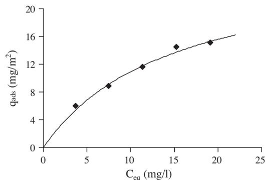
**Figure 5** Adsorption isotherm of RY84 on the photocatalyst.
