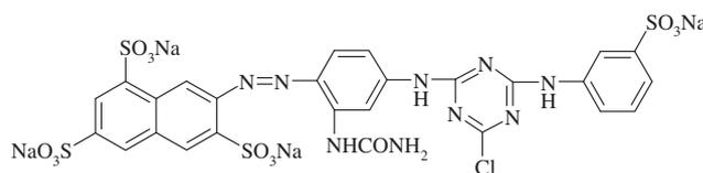
**Figure 1** Chemical structure of Reactive Yellow 84.
