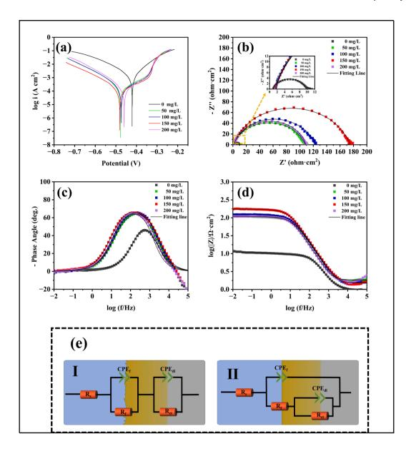
Fig. 6. PDP data result (a), EIS data result (b-d), and fitted circuit
