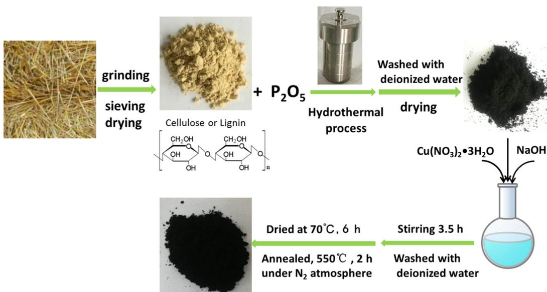
**Scheme 1** Schematic illustration for the synthetic procedure of the catalysts.
