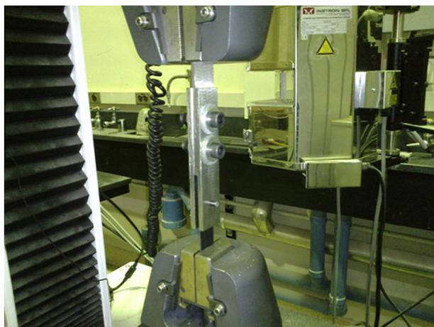
Figure 5 Load bearing test set up.
