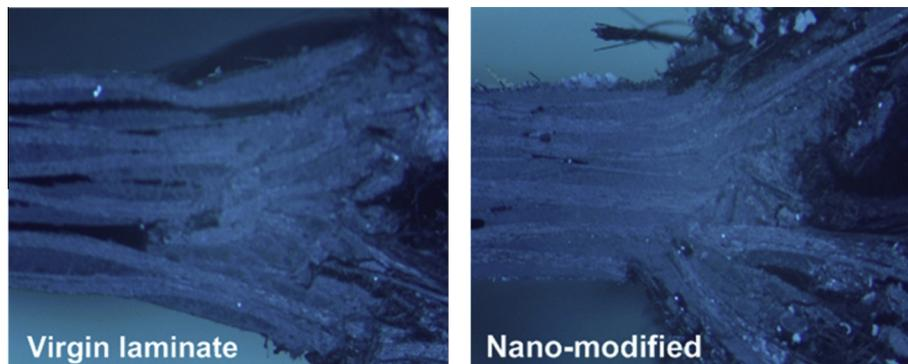
Figure 10 Fracture surface of the cross-section bearing plane.
