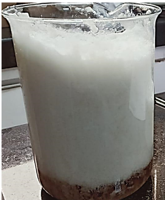
Fig. 7 Effervescence process after addition of PDUE-urea mixture (after retention time of 12 h) to ZrOCl_2 solution.
