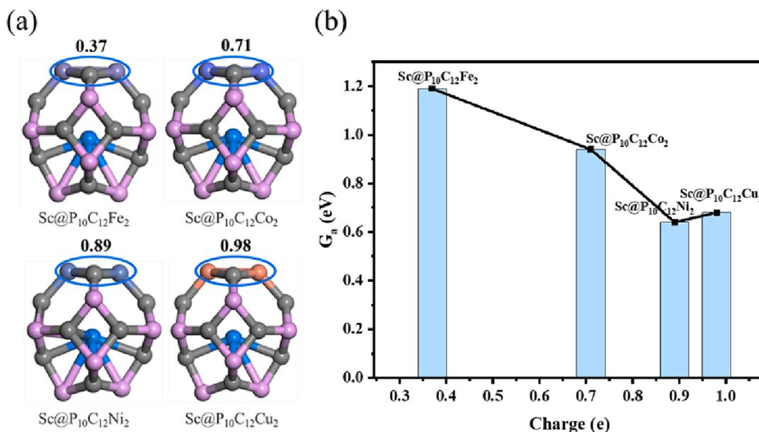
Fig. 6. Charge (e) in the four-membered ring and its relation to the activation free energy of the rate-limiting step on the Sc@P<sub>10</sub>C<sub>12</sub>M<sub>2</sub> catalysts.
