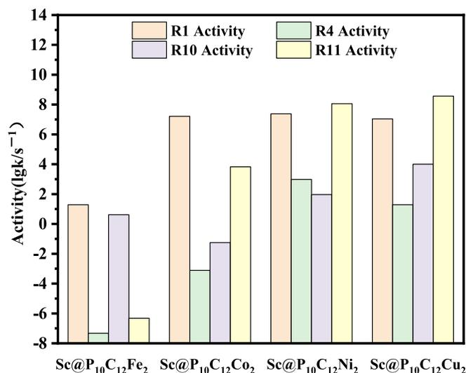
**Fig. 3.** The activity (lgk/s<sup>-1</sup>) of the main pathway of CH<sub>3</sub>OH to CHOOCH<sub>3</sub> on the Sc@P<sub>10</sub>C<sub>12</sub>M<sub>2</sub> catalysts.
