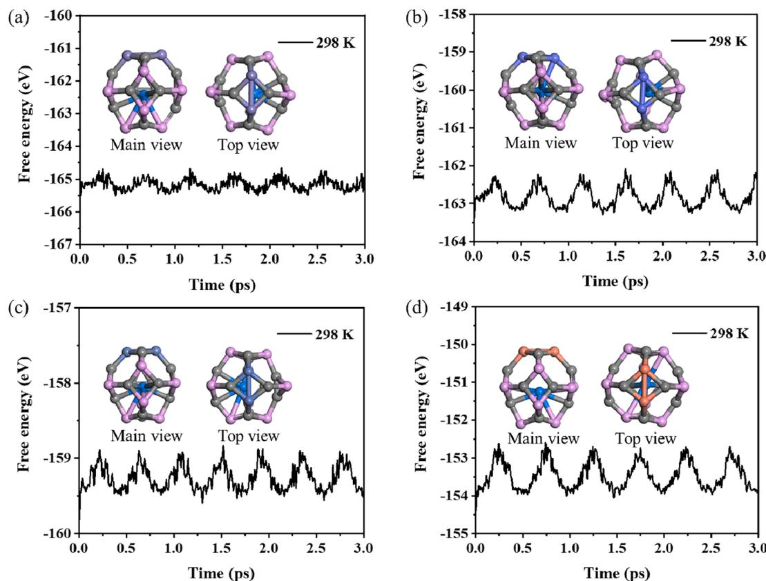
Fig. 2. Total energy fluctuations of Sc@P<sub>10</sub>C<sub>12</sub>M<sub>2</sub> during molecular dynamics simulations and geometry at the end of the simulation.
