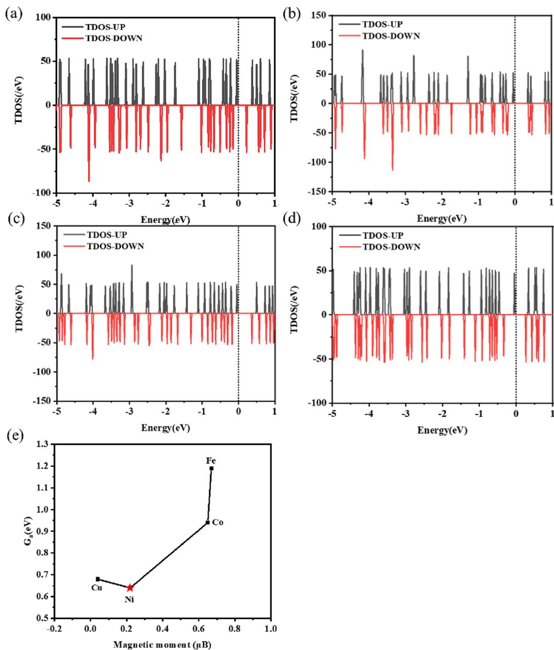
Fig. 4. The density of states of (a) Sc@P<sub>10</sub>C<sub>12</sub>Fe<sub>2</sub>, (b) Sc@P<sub>10</sub>C<sub>12</sub>Co<sub>2</sub>, (c) Sc@P<sub>10</sub>C<sub>12</sub>Ni<sub>2</sub> and (d) Sc@P<sub>10</sub>C<sub>12</sub>Cu<sub>2</sub>. (e) The relationship between the magnetic moment of 2Fe, 2Co, 2Ni, 2Cu and the activation free energy of the rate-limiting step of CH<sub>3</sub>OH to CH<sub>3</sub>OCH<sub>3</sub>.
