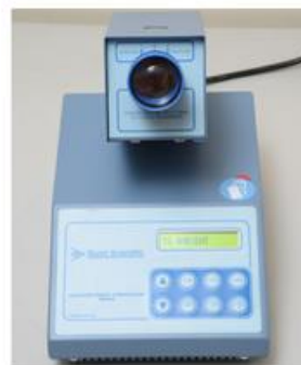
Melting points were determined by using Stuart in 0.5 mm (o.d.) glass capillaries by a SMP3 melting point apparatus.
