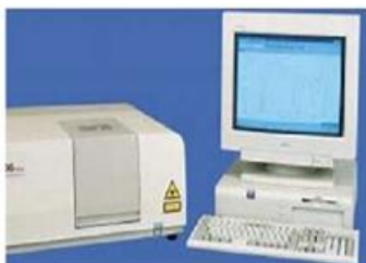
All IR spectra were recorded in KBr discs Shimadzu FT IR 8101 PC IR spectrophotometer.
