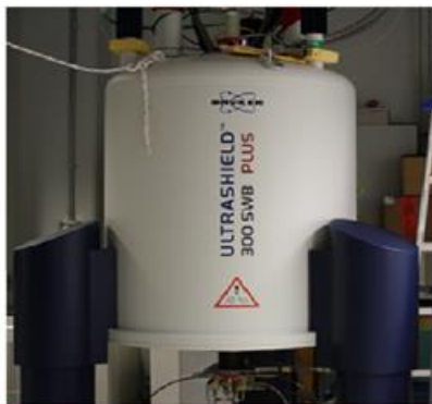
NMR-spectra (Nuclear magnetic resonance spectra) have been determined in deuterated solvent (DMSO- d 6 ) utilizing a Bruker Avance 300 instrument at 300 MHz for 1 H NMR or 75 MHz for 13 C NMR in DMSO- d 6 solutions. The measuring units for \delta and J are ppm and Hz, respectively.
