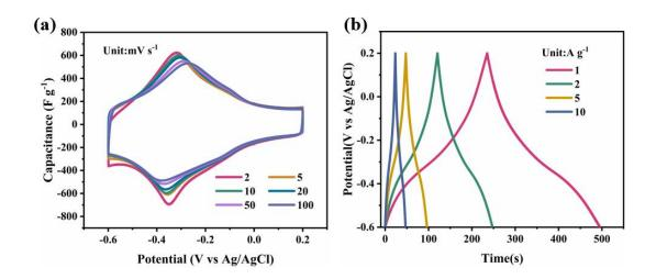
**Fig. S2.** Electrochemical test of  $Ti_3C_2T_x$  electrodes: (a) CV curves of  $Ti_3C_2T_x$  at different scan rates. (b) GCD curves of  $Ti_3C_2T_x$  at different current density.
