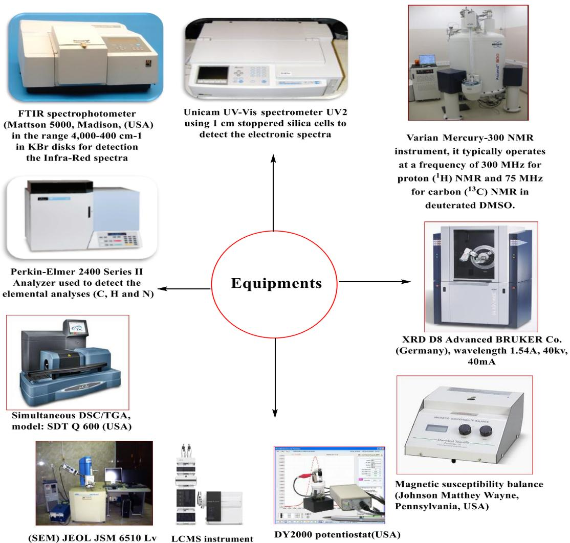
**Scheme 2S.** The Equipment's used for structural characterization
